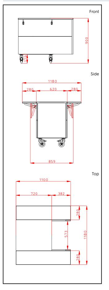
Flexy Compact Cashier Unit with wheels and two stainless steel tray sliders, H=900mm
